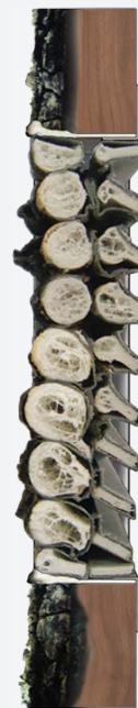
LVN20 air transfer grille in hot condition, showing intumescent material expanding to fill the space in the door
